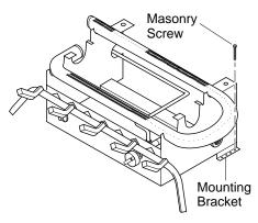
Figure 13 - Attaching Base Assembly to Fireplace Floor - Dual Burner Model
